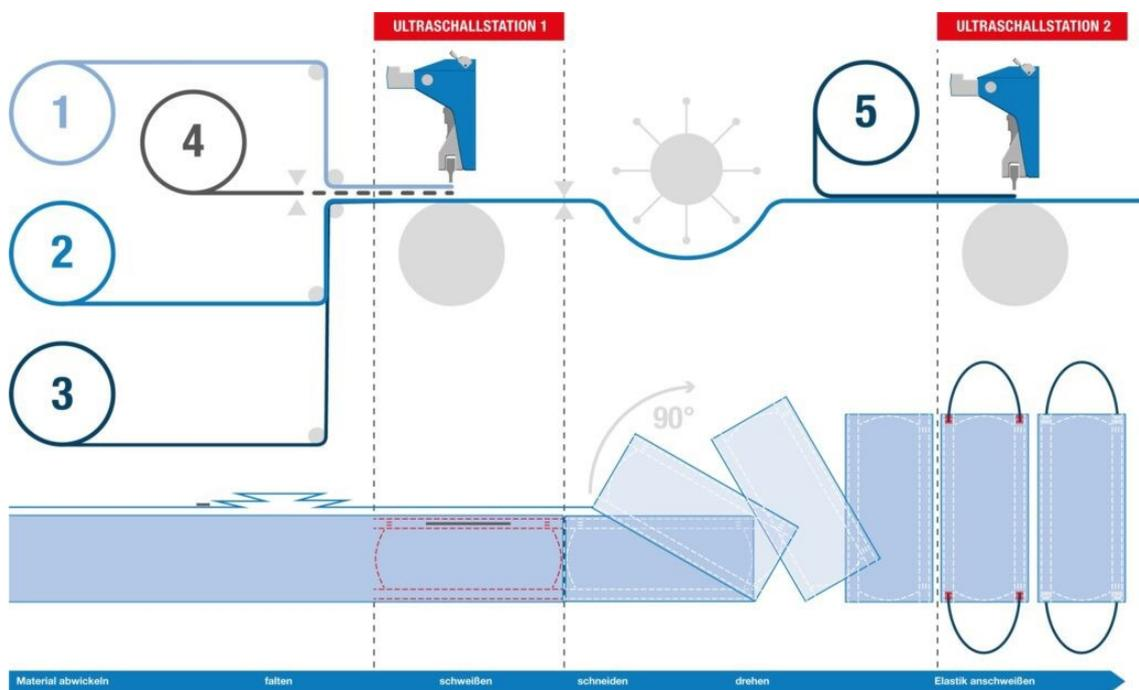
This is how a fully automated production line for flat surgical face masks works. Photo: Herrmann Ultraschalltechnik
